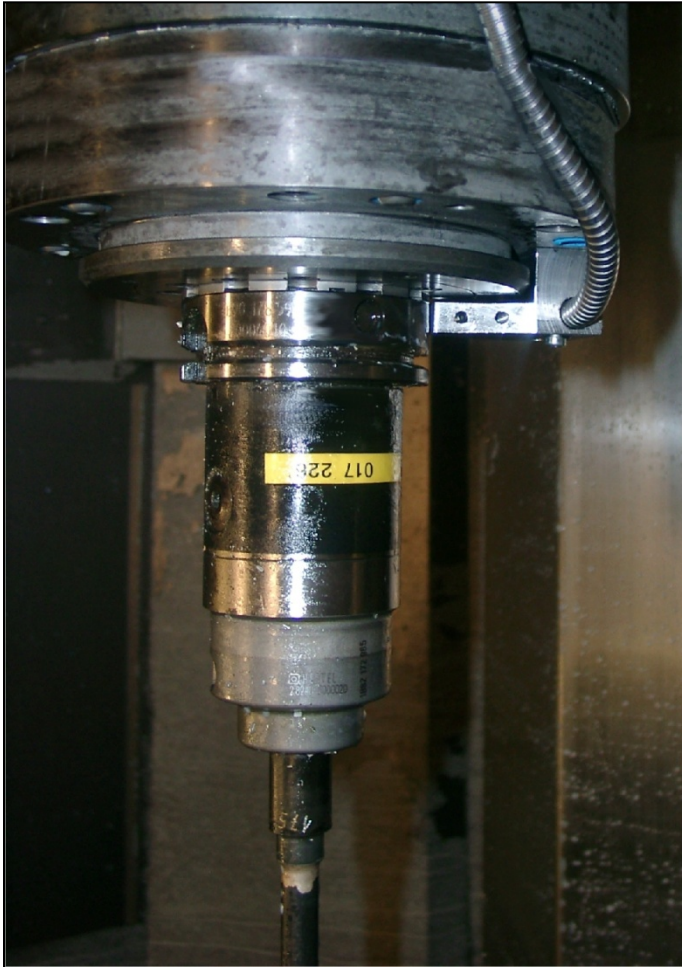
Distance measurement at hollow shaft cone
