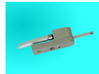
X(Y,Z)-Gauging Element Acoustic detection of friction noise that the rotating grinding wheel generates when touching the diamond surface. Implemented with a diamond surface on a spring steel element as a wave guide. Application: grinding machines (e.g. work piece grinding)
