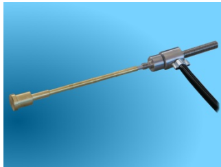
RSA-2 Rotating acoustic emission sensor Rotating piezo-electrical acoustic emission sensor with integrated transmitter. The acoustic emission value is inductively transmitted to a fixed receiver.
