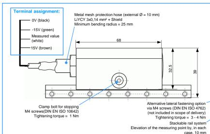
Center of the measuring spherical cap Installation dimensions from the central measurement point of the spherical can
