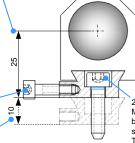
M5 (DIN EN ISO 4762) with breakneck groove (in the scope of delivery) Tightening torque = 4 - 5 Nm
